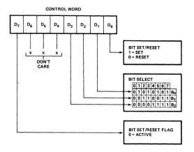
Figure 5. Bit Set/Reset Format
